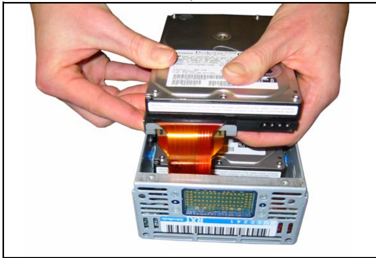
Figure 3-13 Replacing the bracket on the connector.
